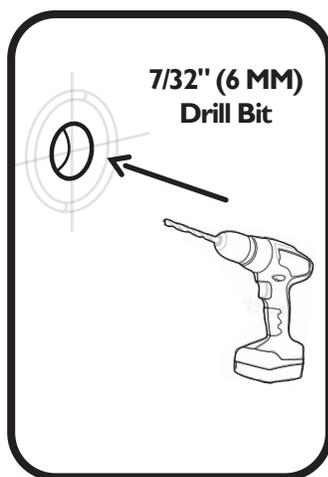
**Step 2A:** Use a 7/32" (6 MM) drill bit to bore the holes on the wall for the anchors, washers and screws provided.
