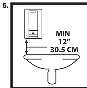
The dispenser should be mounted 12" (30.5 CM) above the counter-top, sink or other surface. If an object remains in the sensing range for more than 10 seconds, the white and green LED will begin blinking and no soap will be dispensed after the initial dose. Remove object and unit will operate normally.
