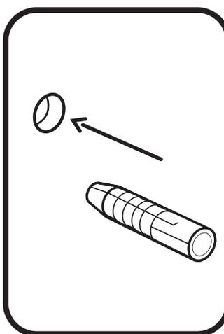
**Step 2B:** Insert anchors into all three holes.
