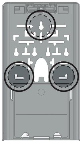
**Step 1:** The Dispenser housing provides numerous mounting locations. If replacing a competitive unit, determine if one (or more) of the holes match.
