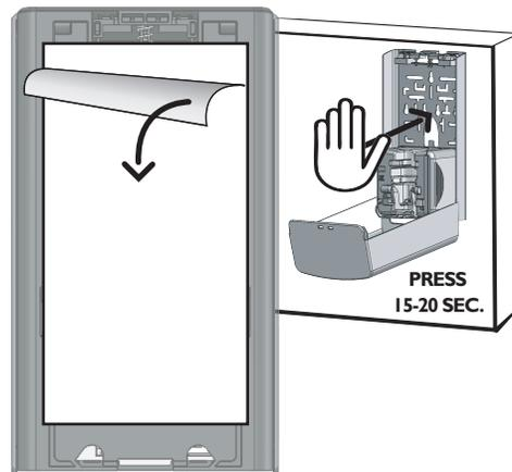
**Step 2:** Remove the red backing from the tape. Ensure that the dispenser is in a level position on the wall, open cover and press the dispenser firmly for 15 to 20 seconds to allow it to properly adhere to wall.
