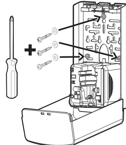
**Step 3:** Insert the washers over the screws and then use a screwdriver to insert the screws in to the anchors and tighten the dispenser securely against the wall.
