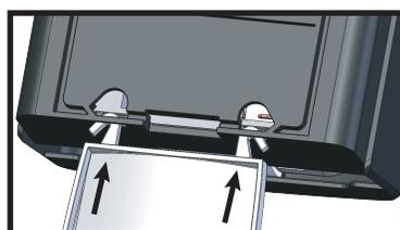
Insert drip catch hooks (a) through rectangular slots located at the bottom rear of the dispenser. The Drip-Catch will SNAP into place.
